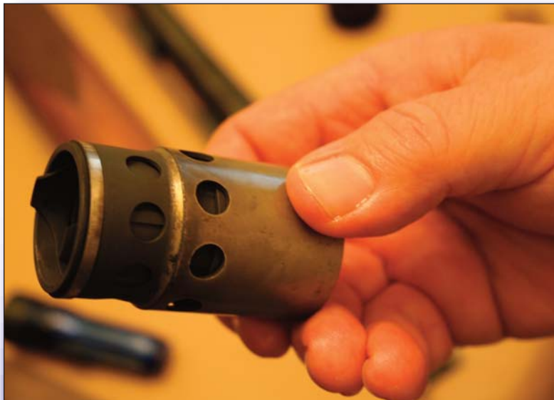
This badly tarnished gas cylinder from John Thompson's 12-gauge shotgun cleaned up nicely in short order when attacked with the chemist's odorless and environmentally friendly gun-cleaning solution.
