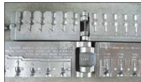
A production mold for making one size head. And another making numerous weights of a jig worm bass head.
