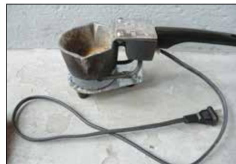
A small melting pot that works quite well.
