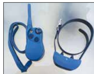
A typical e-collar showing the transmitter on the left and the receiver and collar on the right.
