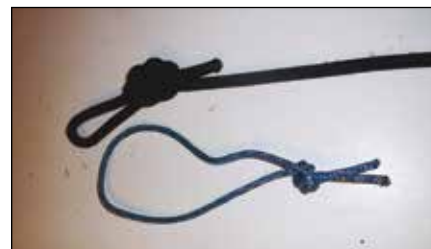
Top: Safety line with overhand knot. Bottom: Loop with overhand knot for Prusik hitch.
